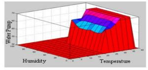
Fig.15. Plot between Temperature-Humidity & Water Pump Speed
