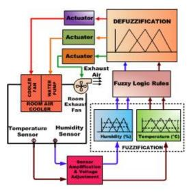
Fig.1. Block diagram of Autonomous Room Air Cooler System
